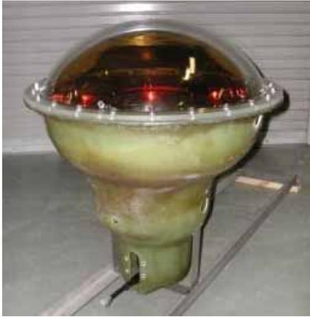
Figure 3.23: Photograph of a 20 inch PMT covered by acrylic and FRP.
